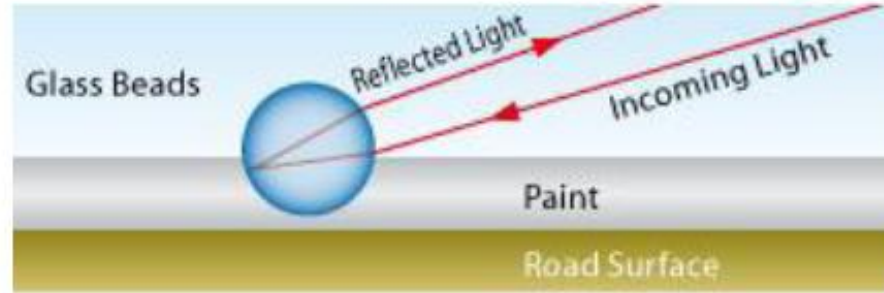
Principle of light reflection in lane markings
